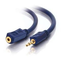
Specifically designed to extend the connection from your PC sound card, portable CD player, MP3 player, iPod, or any mini-stereo audio device to another audio device. This cable features two 27 AWG oxygen-free copper conductors, a drain wire, an aluminum foil shield to prevent unwanted EMI/RFI interference, and fully molded, gold-plated connectors providing strain relief for a quality connection.
